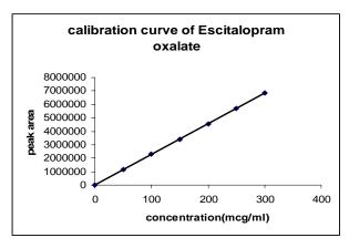
Fig. 1: Calibration curve Escitalopram oxalate
