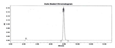
Fig. 3: Chromatogram of Sample Escitalopram
