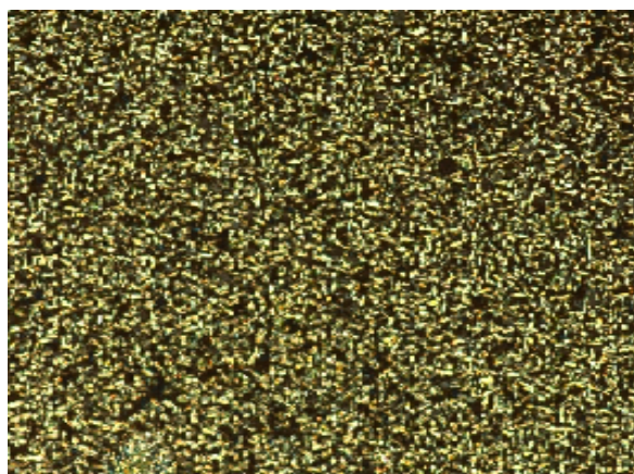
Fig. 5: Photomicrographs of the optical textures of M phase mesophases obtained just below the isotropic liquid phase of 16alddd
